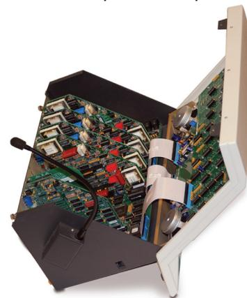
The Console operates from 12 Volts DC, which is available from Zetron's universal power-supply that accepts any voltage from 95 to 250 VAC at 47 to 440 Hz. The universal power-supply has UL, CSA and VDE approvals.
